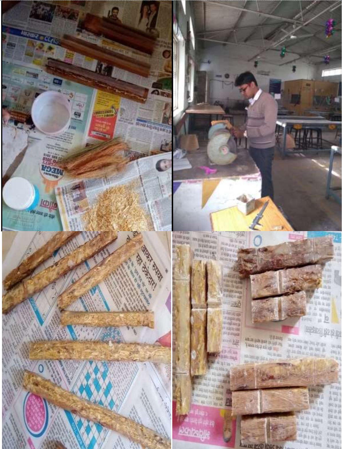
Figure 2.3 Open mould system used for making composites & Sample Preparation
